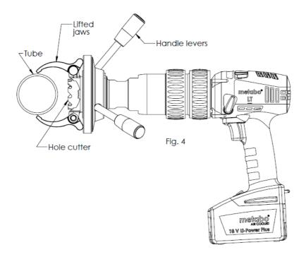
4. Referring to fig. 4, loosen the jaws by rotating the thrust lock nut anticlockwise. The torsion springs will lift up the jaws thus enable the snap drill to be pulled free.
