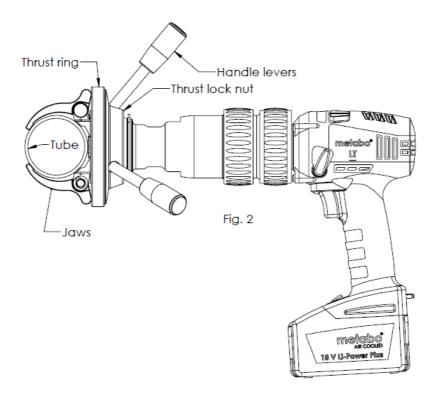
2. Referring to fig. 2, fasten the snap drill to the tube by tightening the jaws against the tube by rotating the thrust lock nut clockwise against the thrust ring by the help of the handle levers.
