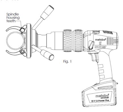
1. Referring to fig. 1, place the teeth in the spindle housing against the tube where to drill the hole.
