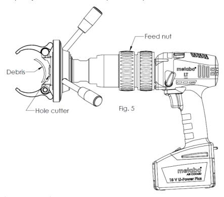
5. Referring to fig. 5, get rid of the debris by rotating the drill anticlockwise and gently rotate the feed nut outwards to engage the clutch. The hole cutter will now move backwards pushing the debris against the hexagon drive shaft thus throwing it free from the hole cutter.
