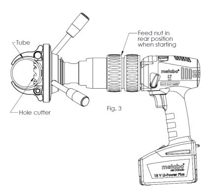
3. Referring to fig. 3, check that the feed nut is in the rear position before start. Lubrication directly in the hole saw ahead of drilling is recommended. Start the battery drill clockwise pushing the button fully down to achieve full torque. Use battery drill gear stage 2 for hole cutters up to and included Ø30 mm, and gear stage 1 larger than Ø30 mm. Gently rotate the feed nut outwards to engage the clutch. The hole cutter will now move outwards and cut the hole in the tube.
