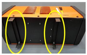
4 Mount and fix the water cooler to the base unit (item 1) using the supplied qty 4 screws (B).
