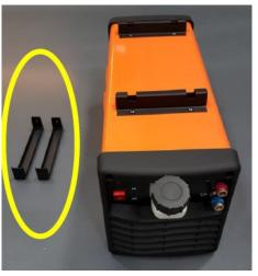
Place the cooler on its side and mount the two brackets supplied with the water cooler (circled yellow) to the bottom of the cooler as shown using the screws (B) supplied with the cooler.
