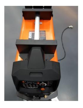
9 Mount the top shelf (item 2) on top of the fitted brackets and use the screws removed earlier to fix the top shelf in place. Also secure the top shelf (item 2) to the cylinder upright (item 3) with screws (A).
