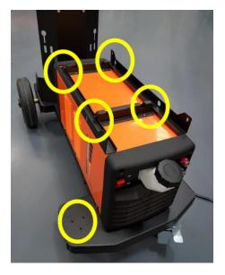
6 Fit the TIG wire 'cup' (item 5) to the base using the supplied 3 screws (C)
