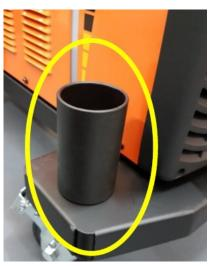
7 Remove the bottom side front and rear screws either side of the power source (the middle screw may not be required to be removed) and mount the power source on top of the water cooler lining up the holes of the bracket. (The bracket should be on the outside of the power source panel). Secure the power source with the screws that were removed.
